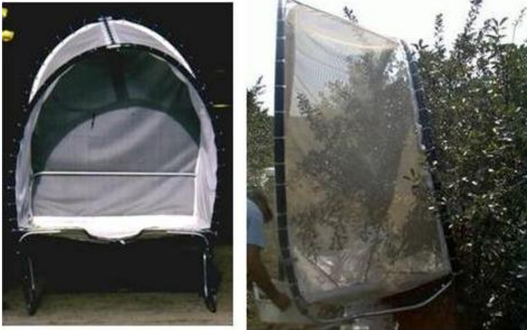
Figure 1. Photo of catch frame showing front and side views. There is no need for the front part to be shorter than the back. We could have trimmed that back part to be the same height.
